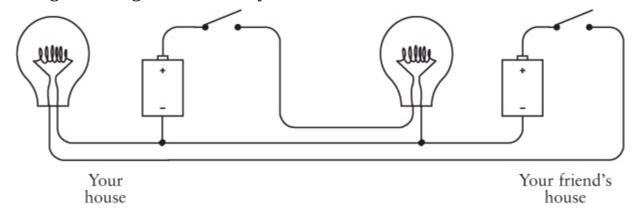
Notice that the negative terminals of the two batteries are now connected. The two circular circuits (battery to switch to bulb to battery) still operate independently, even though they're now joined like Siamese twins.
