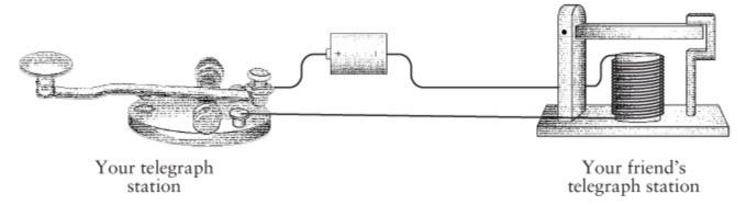
As we discovered, you don't need two wires connecting the two telegraph stations. One wire will suffice if the earth provides the other half of the circuit.
