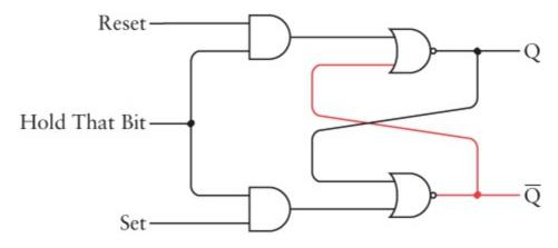
Recall that the output of an AND gate is 1 only if both inputs are 1. In this diagram, the Q output is 0 and the  $\overline{\mathbb{Q}}$  output is 1.
