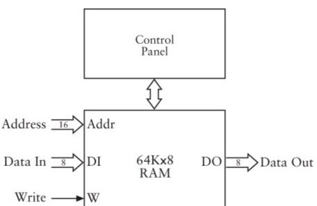
If you had typed all 100 binary numbers into this RAM array rather than directly into the adding machine, making a few corrections would be a lot easier.
