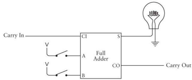
The carry output from the first Full Adder is an input to this second Full Adder. Each subsequent
