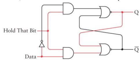
The Q output is now the same as the Data input, and <sup>Q</sup> is the opposite. Now Hold That Bit can go back to being 0:
