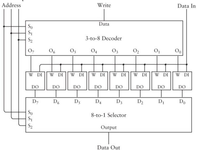
Notice that the three Select signals to the Decoder and the Selector are the same and that I've also labeled those three signals the *Address*. Like a post office box number, this 3-bit address determines
