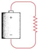
The squiggly line is recognizable to electrical engineers as the symbol for a resistor. Here it means that the circuit has a resistance that is neither very low nor very high.
