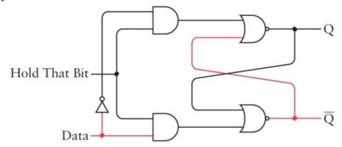
But when Hold That Bit is 1, the circuit reflects the value of the Data input:
