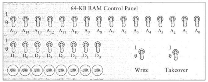
All the switches are shown in their off (0) positions. I've also included a switch labeled *Takeover*. The purpose of this switch is to let other circuits use the same memory that the control panel is connected to. When the switch is set to 0 (as shown), the rest of the switches on the control panel don't do anything. When the switch is set to 1, however, the control panel has exclusive control over the memory.
