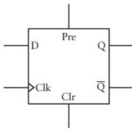
You'll recall that the Preset and Clear inputs should both be 0 for normal operation. But if Preset is 1, Q becomes 1. And if Clear is 1, Q becomes 0.
