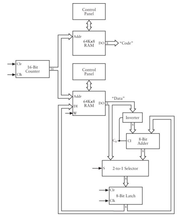
Now suppose we wish to add 56h and 2Ah together and then subtract 38h from the sum. You can do it with the following codes and data stored in the two RAM arrays:
