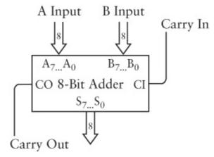
The double-line arrows have an 8 inside to indicate that each represents a group of eight separate signals. They are labeled  $A_7...A_0$ ,  $B_7...B_0$ , and  $S_7...S_0$  also to indicate 8-bit numbers.
