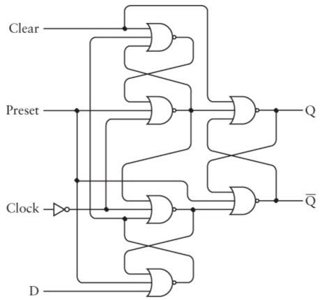
The Preset and Clear inputs override the Clock and Data inputs. Normally these two inputs are 0. When the Preset input is 1, Q becomes 1 and  $\overline{\mathbb{Q}}$  becomes 0. When the Clear input is 1, Q becomes 0 and  $\overline{\mathbb{Q}}$  becomes 1. (Like the Set and Reset inputs of an R-S flip-flop, Preset and Clear shouldn't be 1 at the same time.) Otherwise, this behaves like a normal edge-triggered D-type flip-flop:
