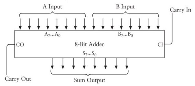
This is a common way to label the separate bits of a multibit number. The bits  $A_0$ ,  $B_0$ , and  $S_0$  are the
