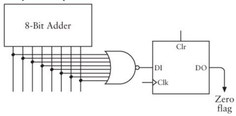
The output of that 8-bit NOR gate is 1 only if all the inputs are 0. Like the Clock input of the Carry latch, the Clock input of the Zero latch latches a value only when an *Add*, *Subtract*, *Add with Carry*, or *Subtract with Borrow* instruction is being performed. This latched value is known as the *Zero flag*. Watch out because it could seem as if it's working backward: The Zero flag is 1 if the output of the adder is all zeros, and the Zero flag is 0 if output of the adder is not all zeros.
