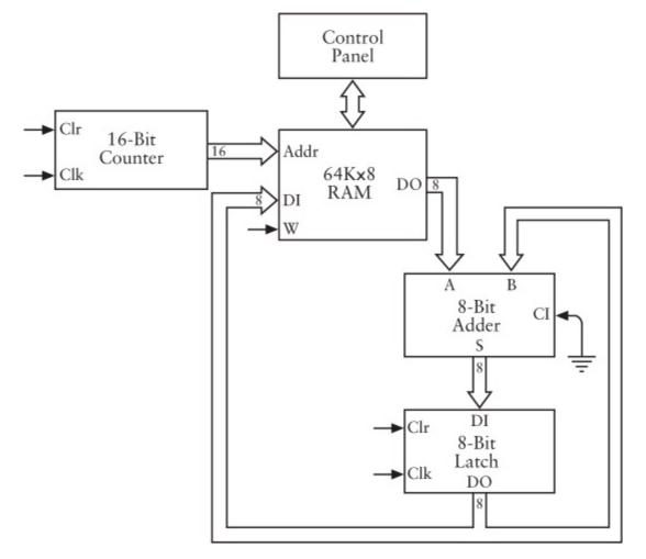
I've eliminated some other parts of the automated adder in this diagram as well, specifically the oscillator and the Clear switch. I removed them because it's no longer at all obvious where the Clear and Clock inputs to the counter and the latch will come from. Moreover, now that we've made use of the RAM data inputs, we need a way to control the RAM Write signal.
