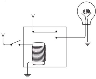
When the switch is closed, a current flows between V and ground through the coils of the electromagnet. This causes the electromagnet to pull the flexible metal contact. That connects the circuit between V, the lightbulb, and ground. The bulb lights up:
