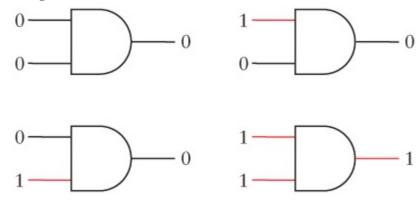
As with the two switches wired in series, the AND gate can also be described in this little table:
