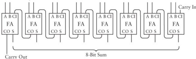
Here's the complete 8-Bit Adder drawn as one box. The inputs are labeled  $A_0$  through  $A_7$  and  $B_0$  through  $B_7$ . The outputs are labeled  $S_0$  through  $S_7$  (for sum):
