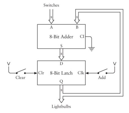
Notice that the switch labeled *Add* now controls the Clock input of the latch.
