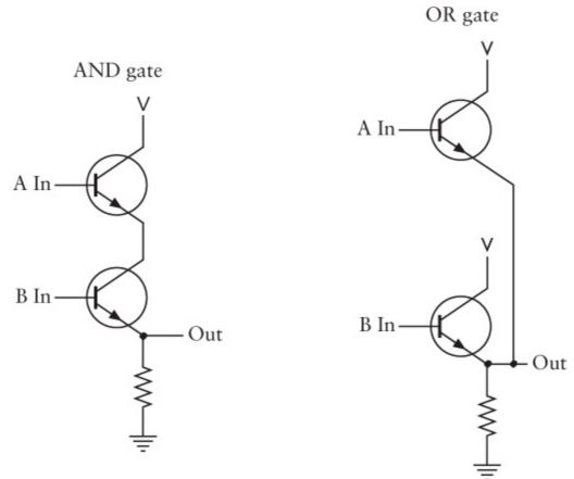
So everything we learned about constructing logic gates and other components from relays is valid for transistors. Relays, tubes, and transistors were all initially developed primarily for purposes of amplification but can be connected in similar ways to make logic gates out of which computers can be built. The first transistor computers were built in 1956, and within a few years tubes had been abandoned for the design of new computers.
