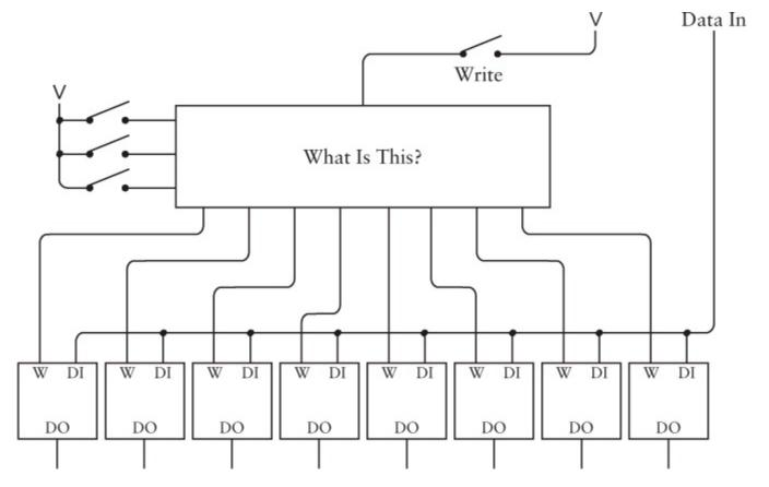
To accomplish this task, we need another circuit that looks somewhat similar to the 8-to-1 Selector but actually does the opposite. This is the *3-to-8 Decoder*. We've also seen a simple Data Decoder before—when wiring the switches to select the color of our ideal cat in Chapter 11.
