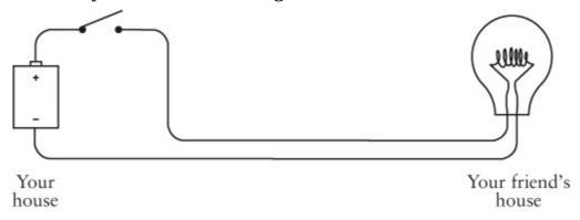
Although I'm showing only one battery, you might actually be using two. In this and future diagrams, this will be an off (or open) switch:
