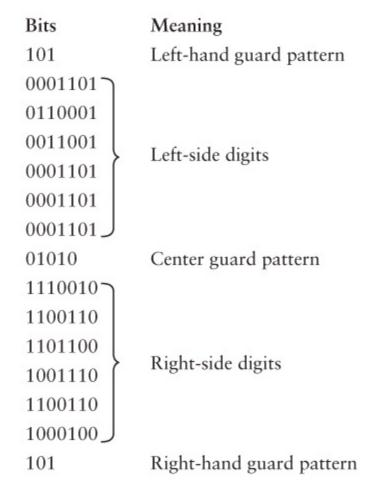
The first 3 bits are always 101. This is known as the *left-hand guard pattern*, and it allows the computer-scanning device to get oriented. From the guard pattern, the scanner can determine the width of the bars and gaps that correspond to single bits. Otherwise, the UPC would have to be a specific size on all packages.
