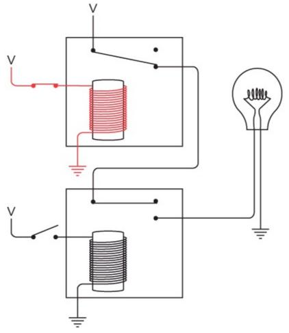
Still the lightbulb doesn't light because the bottom switch is still open and that relay isn't triggered. We can try opening the top switch and closing the bottom switch:
