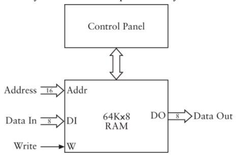
When the Takeover switch is closed, you can use the 16 Address switches to select any of 65,536 addresses. The lightbulbs show you the 8-bit value currently stored in memory at that address. You can use the 8 Data switches to define a new value, and you can write that value into memory using the Write switch.
