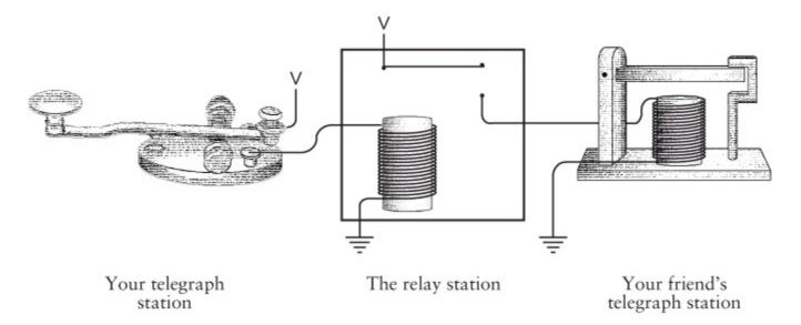
The relay is a remarkable device. It's a switch, surely, but a switch that's turned on and off not by human hands but by a current. You could do amazing things with such devices. You could actually assemble much of a computer with them.
