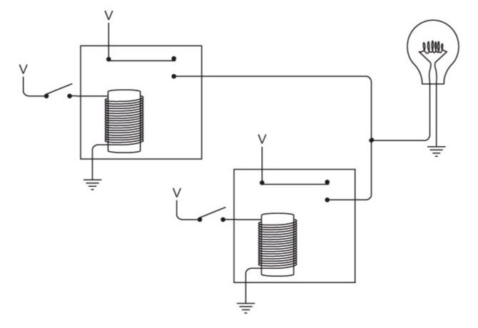
Notice that the outputs of the two relays are connected to each other. This connected output then provides power for the lightbulb. Either one of the two relays is enough to light the bulb. For example, if we close the top switch, the bulb lights up. The bulb is getting power from the left relay.
