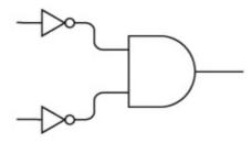
Two inputs are inverted and become inputs to an AND gate. Sometimes a configuration like this is drawn without the inverters:
