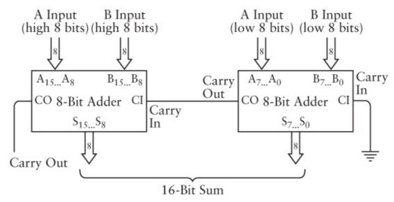
The Carry Out of the adder on the right is connected to the Carry In of the adder on the left. The adder on the left has as input the most-significant eight digits of the two numbers to be added and creates as output the most-significant eight digits of the result.
