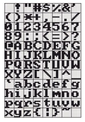
These are the characters corresponding to ASCII codes 20h through 7Fh. (No visible characters are associated with ASCII codes 00h through 1Fh.)
