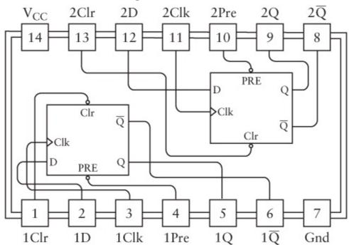
The TTL Data Book even includes a logic diagram for each flip-flop in this chip:
