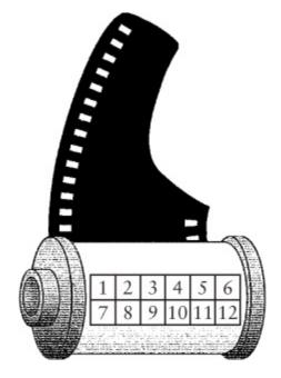
You'll see a checkerboard-like grid of silver and black squares that I've numbered 1 through 12 in the diagram. This is called *DX-encoding*. These 12 squares are actually 12 bits. A silver square means a 1 bit and a black square means a 0 bit. Square 1 and square 7 are always silver (1).
