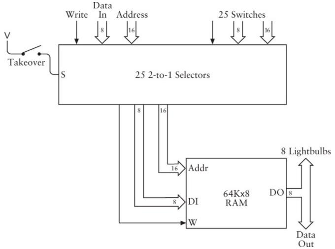
When the Takeover switch is open (as shown), the Address, Data input, and Write inputs to the  $64K\ x$
