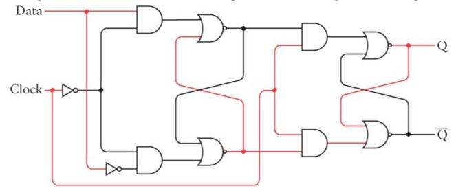
This causes the second stage to change, and the Q output goes to 1. The difference is that the Data input can now change (for example, back to 0) without affecting the Q output:
