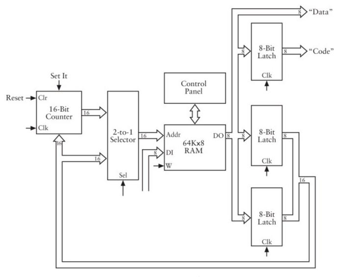
Obviously, we must ensure that the Set It signal is 1 only if the instruction code is 30h and the address has been latched.
