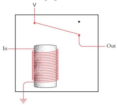
So a telegraph key, a relay, and a sounder are connected more or less like this:
