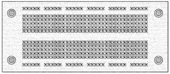
Each short row of 5 holes is electrically connected underneath the plastic base. You insert chips into the breadboard so that a chip straddles the long central groove and the pins go into the holes on either side of the groove. Each pin of the IC is then electrically connected to 4 other holes. You connect the
