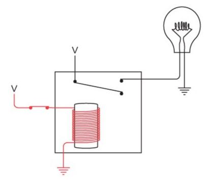
Using the terminology of switches, this type of relay is called a *double-throw* relay. It has two outputs that are electrically opposite—when one has a voltage, the other doesn't.
