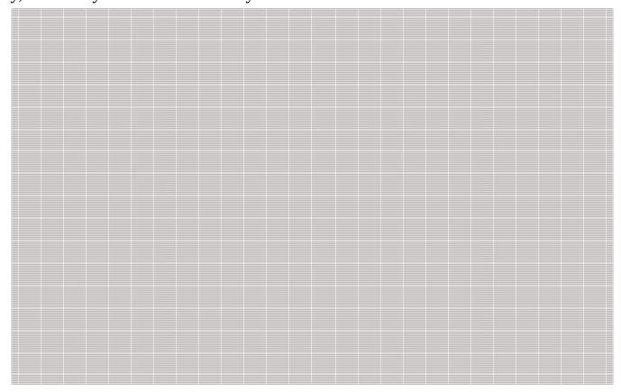
To determine the total number of pixels in this grid, you can count them or simply multiply 320 by 200 to get 64,000 pixels. Depending on how you've configured your video adapter (as I'll explain shortly), each pixel can be either black or white, or each pixel can be a particular color.
