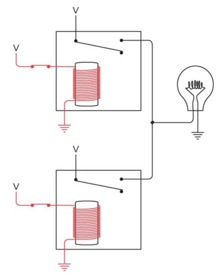
This behavior is exactly opposite that of the AND gate. This is called *NOT AND* or, more concisely, *NAND*. The NAND gate is drawn just like the AND gate but with a circle at the output, meaning the output is the inverse of the AND gate:
