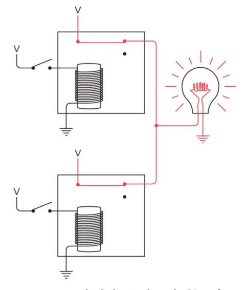
In this case, the two outputs are connected, which is similar to the OR configuration but using the other contacts. The lightbulb is on when both switches are open.
