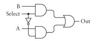
If the Select input is 1, the output of the OR gate is the same as the B input. That's because the output of the top AND gate is the same as the B input, and the output of the bottom AND gate is 0. Similarly, if the Select input is 0, the output is the same as the A input. This is summed up in the following function table:
