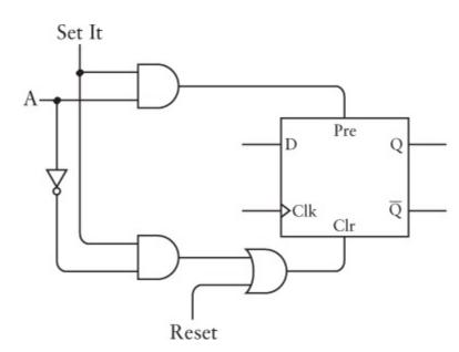
Normally the Set It signal is 0. In that case, the Preset input to the flip-flop is 0. The Clear input is also 0 unless the Reset signal is 1. This allows the flip-flop to be cleared independently of the Set It signal. When the Set It signal is 1, the Preset input will be 1 and the Clear input will be 0 if A is 1. If A is 0, the Preset input will be 0 and the Clear input will be 1. This means that Q will be set to the value of A.
