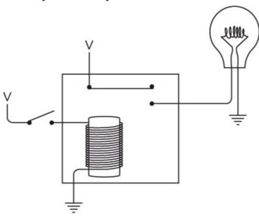
When the switch is closed, the bulb lights up.
