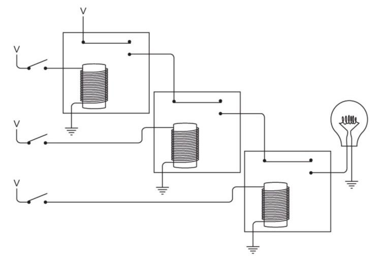
The lightbulb lights up only if all three switches are closed. This configuration is expressed by this symbol:
