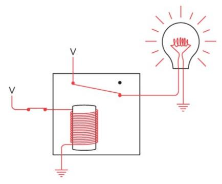
These diagrams of the relay show two voltage sources and two grounds, but in all the diagrams in this chapter, all the V's can be connected to one another and all the grounds can be connected to one another. All the networks of relays and logic gates in this chapter and the next will require only one battery, although it might need to be a big battery. For example, the preceding diagram can be redrawn with only one battery like this:
