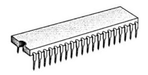
Of course, what you see is just the packaging. The actual wafer of silicon inside is much smaller—in the case of the early 8-bit microprocessors, the silicon is less than ¼ inch square. The packaging protects the silicon chip and also provides access to all of the chip's input and output points through the pins. The diagram on the following page shows the function of the 40 pins of the 8080.
