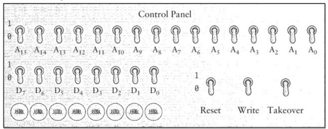
Unlike the earlier control panel, this one has a switch labeled Reset. The Reset switch is connected to the Reset input of the microprocessor. As long as that switch is on, the microprocessor doesn't do anything. When you turn off the switch, the microprocessor begins executing machine code.
