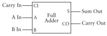
The following table summarizes all the possible combinations of inputs to the Full Adder and the resultant outputs:
