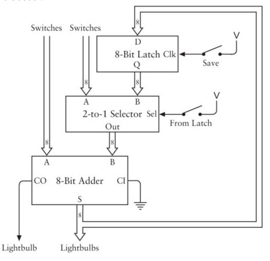
The box labeled 2-Line-to-1-Line Selector lets you choose with a switch whether you want the B inputs to the adder to come from the second row of switches or from the Q outputs of the latches. You close the switch to select the outputs from the 8-Bit Latch. The 2-Line-to-1-Line Selector uses eight of the following circuits:
