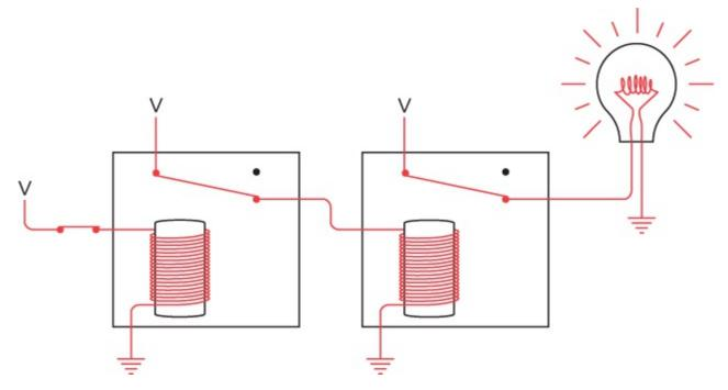
Connecting relays is the key to building logic gates.
