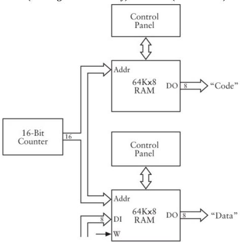
We've already established that our new automated adder needs to be able to write sums into the original RAM array (labeled *Data*). But the new RAM array (labeled *Code*) will be written to solely through the control panel.
