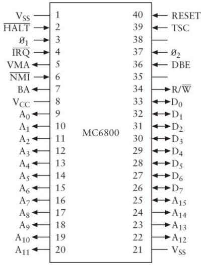
The  $V_{SS}$  indicates Ground, and  $V_{CC}$  is 5 volts. Like the 8080, the 6800 has 16 output Address signals
