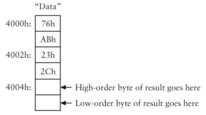
These six locations don't have to be all together like this. They can be scattered anywhere throughout the whole 64-KB Data RAM array. To add these values at these memory locations, you must set up the instructions in the Code RAM array, like this:
