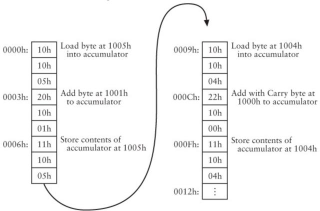
At the completion of these six instructions, the 16-bit value at memory locations 1004h and 1005h will equal A7h times 1. Therefore, these six instructions have to be repeated 27 more times in order for that 16-bit value to equal A7h times 1Ch. You can achieve this by typing in these six instructions 27 more times beginning at address 0012h. Or you can put a *Halt* instruction at 0012h and press the Reset button 28 times to get the final answer.
