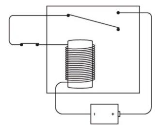
But when the contact changes position, the circuit is no longer complete, so the electromagnet loses its magnetism and the flexible contact flips back up:
