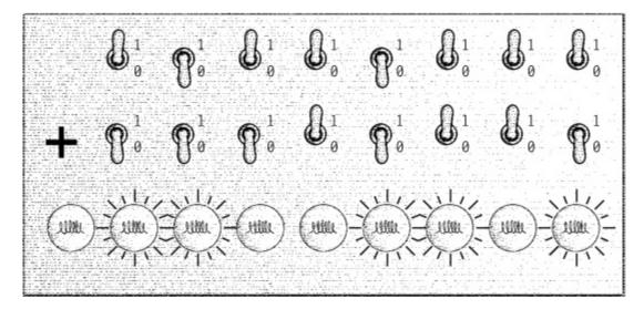
In this diagram, the switches are set to add 183 (or 10110111) and 22 (00010110), producing the result of 205, or 11001101 as shown in the row of lightbulbs.
