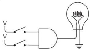
Notice that this symbol for the AND gate not only takes the place of two relays wired in series, but it also implies that the top relay is connected to a voltage, and both relays are connected to ground. Again, the lightbulb lights up only if both the top switch *and* the bottom switch are closed. That's why it's called an *AND gate*.
