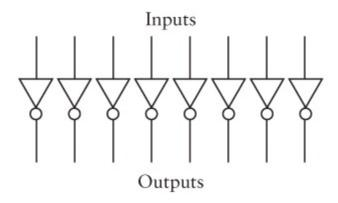
The problem with this circuit is that it *always* inverts the bits that enter into it. We're trying to create a machine that does both addition and subtraction, so the circuitry needs to invert the bits only if a subtraction is being performed. A better circuit looks like this:
