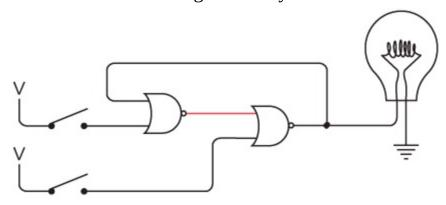
We're back where we started. At this time, you can close and open the bottom switch with no further effect on the lightbulb. In summary
