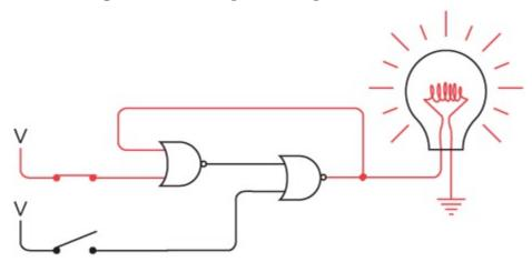
The magic occurs when you now open the upper switch. Because the output of a NOR gate is 0 if either input is 1, the output of the left NOR gate remains the same and the light remains lit:
