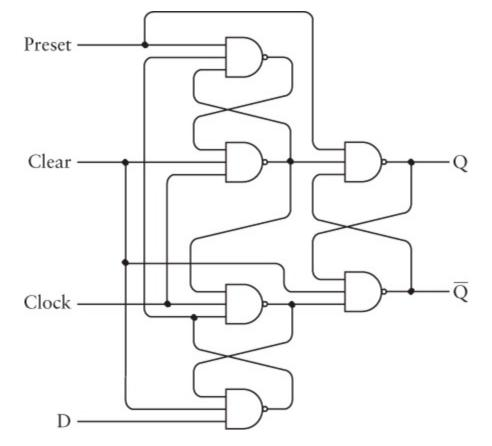
You'll recognize this as being similar to the diagram at the end of Chapter 14, except that I used NOR gates. The logic table in the *TTL Data Book* is a little different as well:
