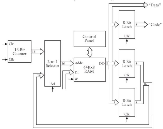
We've made a lot of progress. Now it's possible to enter the instructions and the data in a single RAM array. For example, the diagram on the next page shows how to add two 8-bit numbers together and subtract a third.
