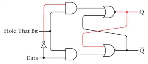
This circuit is called a *level-triggered D-type flip-flop*. The *D* stands for *Data*. *Level-triggered* means that the flip-flop saves the value of the Data input when the Hold That Bit input is at a particular *level*, in this case 1. (We'll look at an alternative to level-triggered flip-flops shortly.)
