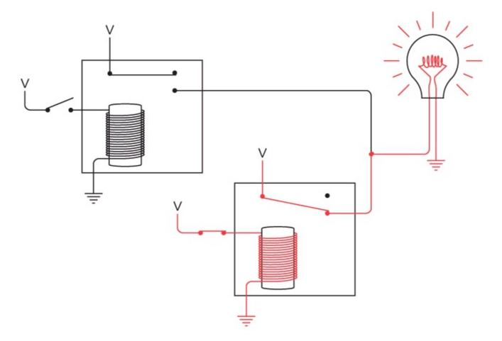
The bulb also lights if both switches are closed:
