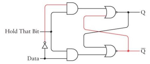
In this case, both inputs are 0 and the output Q is 0 (which means that <sup>Q</sup> is 1). As long as Hold That Bit is 0, the Data input has no effect on the circuit:
