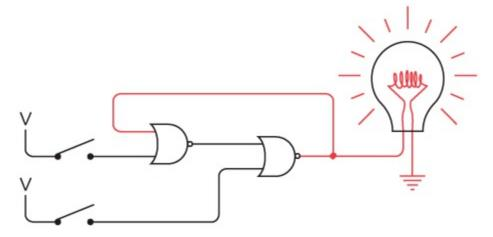
Now this is odd, wouldn't you say? Both switches are open—the same as in the first drawing—yet now the lightbulb is on. This situation is certainly different from anything we've seen before. Usually the output of a circuit is dependent solely upon the inputs. That doesn't seem to be the case here. Moreover, at this point you can close and open that upper switch and the light remains lit. That switch has no further effect on the circuit because the output of the left NOR gate remains 0.
