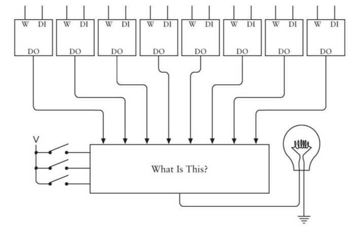
The "something else" is that mysterious box with eight inputs on top and three inputs on the left. By closing and opening the three switches, we can select which of the eight inputs is routed to the output at the bottom of the box. This output lights up the lightbulb.
