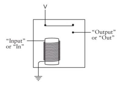
If a current is flowing through the input (for example, if a switch connects the input to V), the electromagnet is triggered and the output has a voltage.
