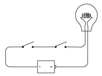
Switches connected in this way—one right after the other—are said to be wired *in series*. If you close the left switch, nothing happens:
