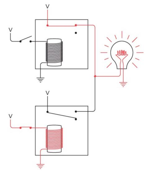
Only when both switches are closed does the lightbulb go off:
