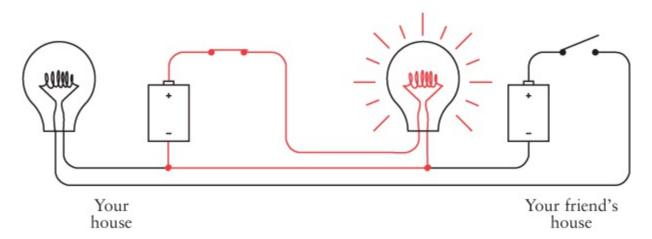
No electricity flows in the other part of the circuit because there's no place for the electrons to go to complete a circuit.
