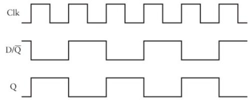
When the Clock input goes from 0 to 1, the value of D (which is the same as  $\overline{Q}$ ) is transferred to Q, thus also changing  $\overline{Q}$  and D for the next transition of the Clock input from 0 to 1.
